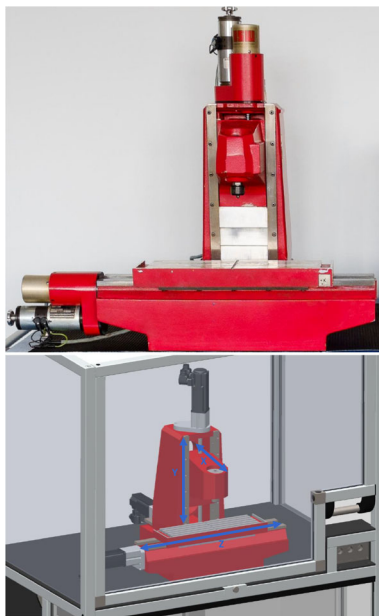
Fig. 3 The 3-axis milling machine for education and demonstration, known as OSACA (above) and its 3D model (below)
