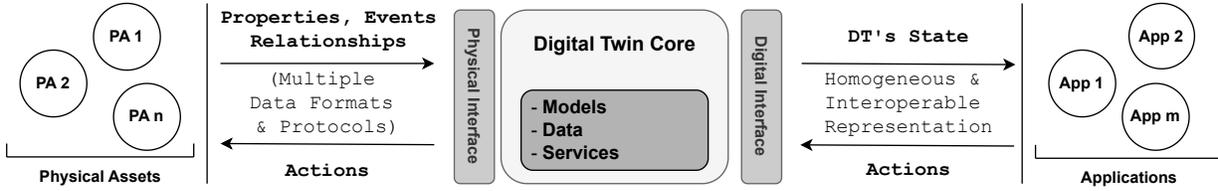
Fig. 2: Abstracted model and structure of a DT with internal components and communication channels.
