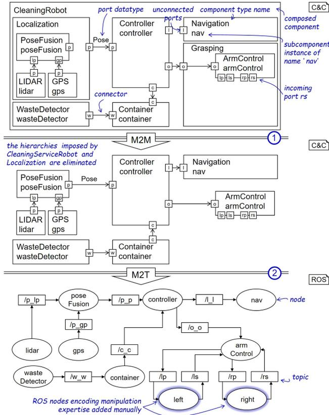
Fig. 2: Component & connector software architecture of a cleaning robot with two arms (top), after applying the M2M transformations for hierarchy elimination (middle), and after applying the M2T transformations producing ROS nodes and topics (bottom).
