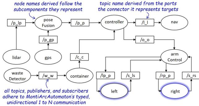
Fig. 18: ROS graph of the cleaning robot architecture depicted in Figure 2.
