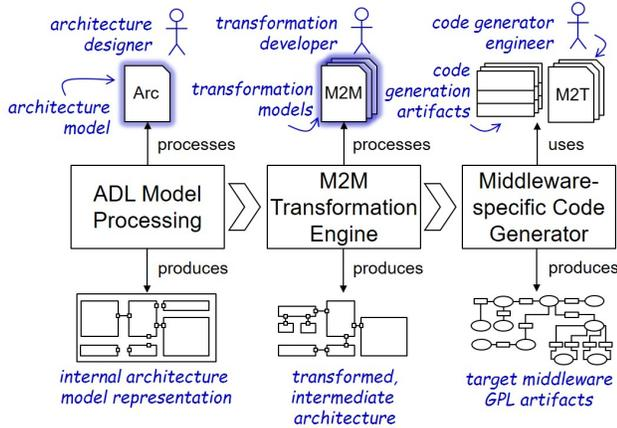
Fig. 1: Quintessential components, artifacts, and roles for pervasive, modular architecture modeling for different target middlewares illustrated on an example of the translation to ROS [6].
